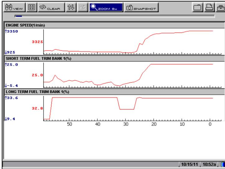
In the capture to the left, the Short Term and Long Term Fuel Trim added together at high RPM is 57.8%, so according to our chart, this is clearly a 'fake' breathing fault. Again, if the engine is really breathing at 28%, it will be fueling for 28% and Fuel Trim will not need to adjust. The fact that this PCM is adding so much fuel indicates that the MAF value is lower than actual engine breathing. If the intake duct isn't disconnected or torn, then it needs a MAF sensor. It just does. Sure, MAF
