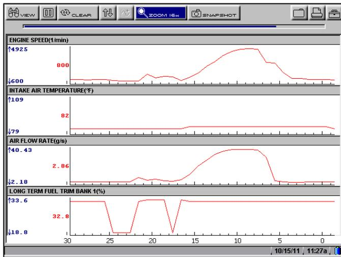
The test drive capture above shows the MAF sensor grams per second, engine speed, and intake air temperature (IAT) during full-throttle acceleration. Long Term Fuel Trim is added in order to make sense of the results (more on that later).
